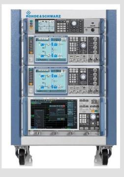
The system consist of Analog SG SMA100A as shared LO, 2 units VSG SMW200A + VNA for time and phase calibration. Plus cables adapters and test bench.
