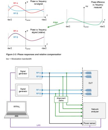
Figure 3-1: RF paths to be aligned
