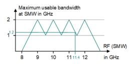
User can not use 2 GHz IQ band at all frequencies in multi-channel mode. Increasing number of calibration points will be time consuming.
