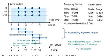
Figure 3-8: Calibration set and relations to the RF signal at the R&S SMW
