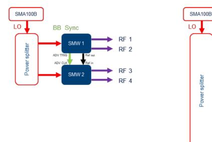
The power splitters need to cover the frequency range from the lowest desired operating frequency (minimum 200 MHz for phase coherence in SMW200A) up to 6.5 GHz (or the highest desired operating frequency, whichever is lower). The most critical signal paths with respect to phase stability are the LO signal distribution (red arrows) the baseband (BB) sync signal distribution (green arrows) and the RF signals (purple arrows).
