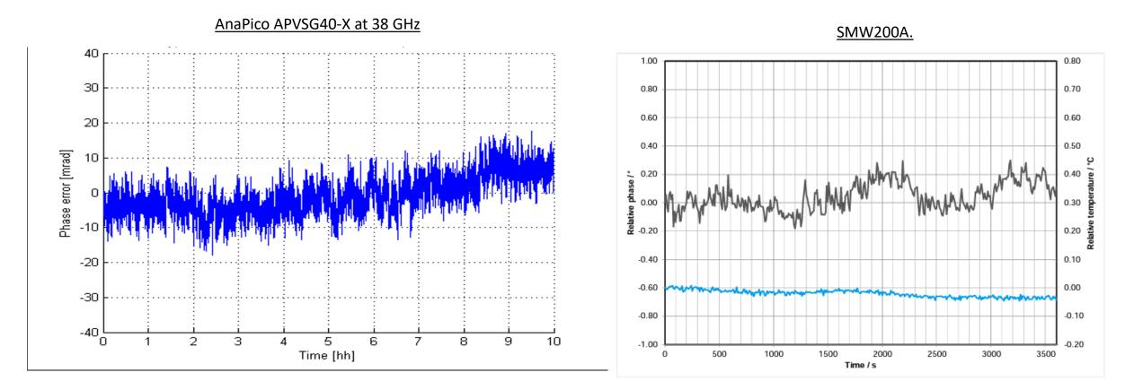
The Maximum amplitude of phase deviation AnaPico APVSG at 38 GHz within 10h 25 mrad is it 1,43 Degree. R&S declares only 1h of operation and with non-realistic temperature stability. In Real conditions 1 deg temperature variations, highly possible that relative phase deviation will be much higher in SMW200A.
