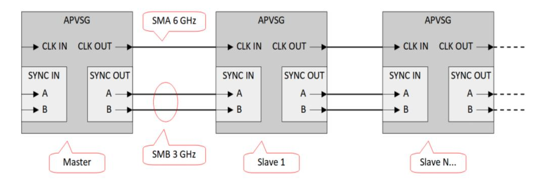
The reference clock uses SMA connectors. Connectors and cable must support at least 6 GHz bandwidth. The synchronization signals A, B, C use SMB connectors. Connectors and cables must support at least 3 GHz bandwidth.
