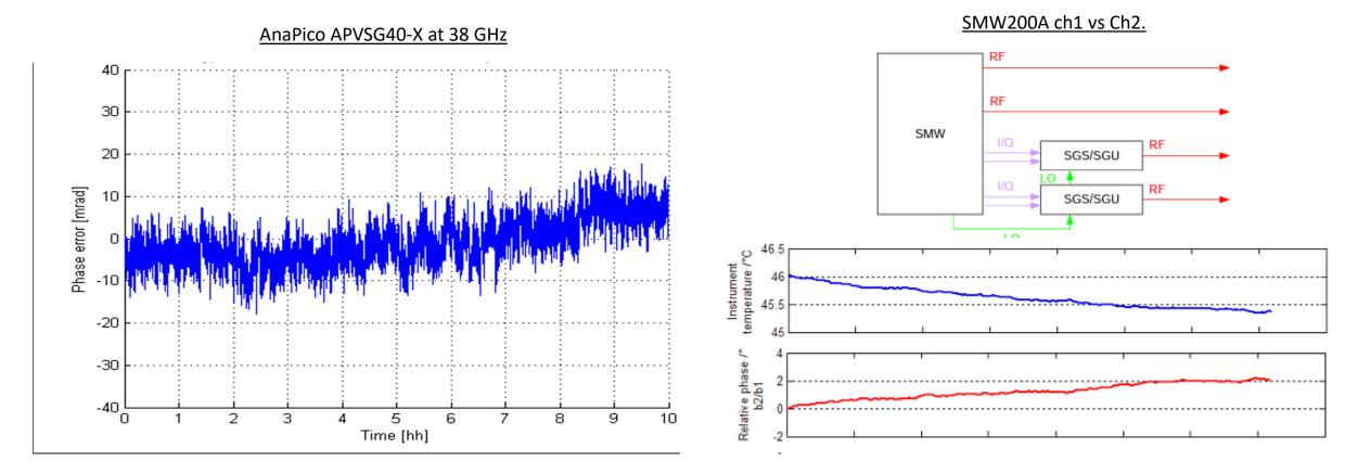
If temperature changed by 0.8 Deg, which is realistic. Relative phase between 2 Channels SMW200A become 2 deg, cascade SMW200A system caused degradation of the relative phase behaviour. AnaPico 4 channels unit has relative phase stability in same temperature conditions <1.5 deg.
